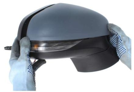
Position the cover onto the mirror unit making sure to line up all of the clips.
