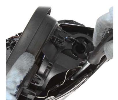
1. Once the mirror cover is removed, locate the screw and using a phillips screwdriver remove the screw.
