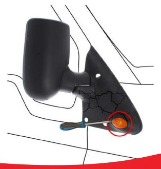
3. Gently pry the side repeater on each side to remove and disconnect so it can be fitted to the replacement unit.
