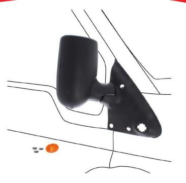
4. Once the old mirror has been removed, reconnect the side repeater and align the replacment unit onto the body.
