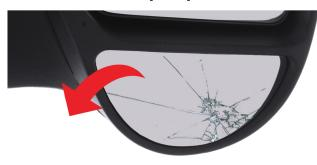
7. Peel off the backing of the new mirror glass and line up with the mirror unit
