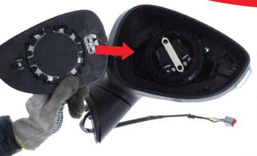
4. Once the heating elements are attached (if needed), line the glass up with the backing plate
