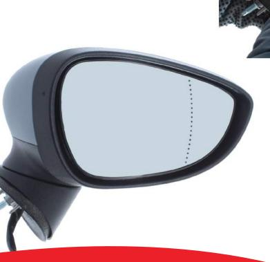
6. Check the glass moves freely and that it isn't loose. Wipe the glass to get rid of any marks
