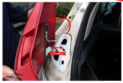
9. To remove the electrical connector, squeeze the clips and pull it towards you.
