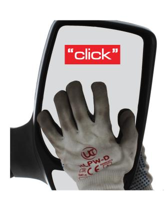
6. Check the glass moves freely and that it isn't loose.Wipe the glass to get rid of any marks
