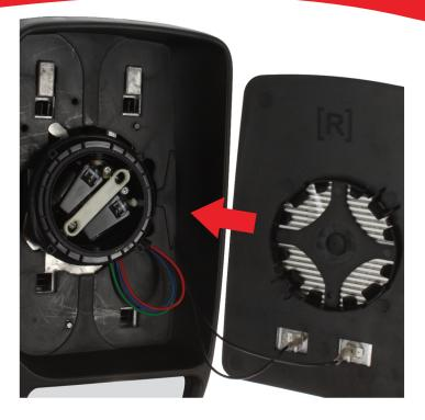
4. Once the heating elements are attached (if needed), line the glass up with the backing plate
