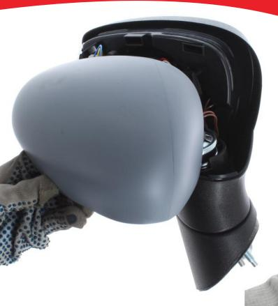
3. Position the cover onto the mirror unit making sure to line up all of the clips
