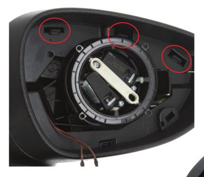
1. Once the mirror glass is removed, carefully pry the clips out of position and pull the mirror cover off.
