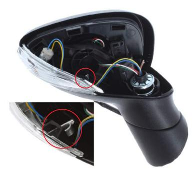
Once the mirror cover is removed, carefully pry the clip out of position and pull the indicator out
