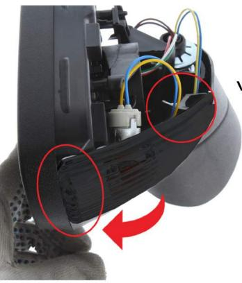
4. Make sure the side of the indicator is lined up with the side of the mirror unit and then the clip.
